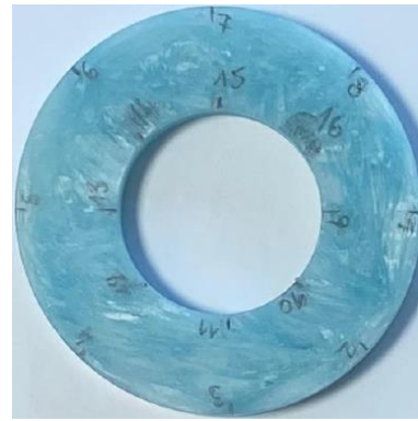
Figure 3: Composite disc with a shaft insert opening - D2.
