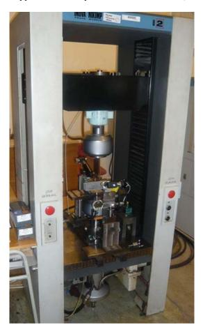
Fig. 4. The three-point bending fatigue test configuration
