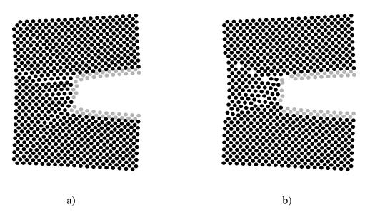
Fig. 5. Dislocations at the left corner of the cavity covered by a thin film of copper atoms at time step  $20\,900h$ ; a) symmetric dislocation emission in the inclined slip systems  $\langle 111 \rangle \{101\}$  on the first two surfaces layers; b) dislocations on the oblique slip planes 112 at the upper corner of the cavity in the middle of the crystal (layers 49–50)
