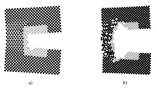
Fig. 6. Detail from the atomic configuration at the Cu nano-inclusion at the left cavity corner in the middle of the crystal (layers 49–50) at time step a) 22400h, b) 24500h
