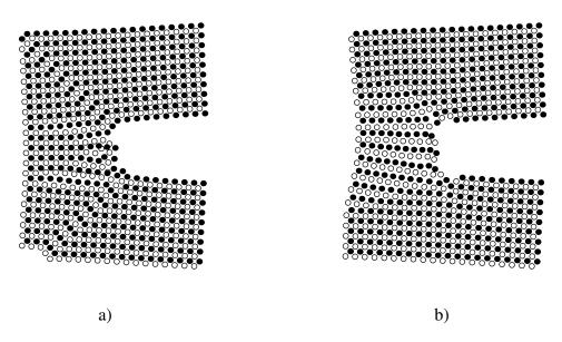
Fig. 3. Detail of the atomic configuration at the left corner of the cavity in pure bcc iron at time step 24500h; a) dislocation emission in the  $\langle 111 \rangle \{101\}$  inclined slip systems, the first two surface layers; b) situation in the layers 43–44 near the middle of the crystal
