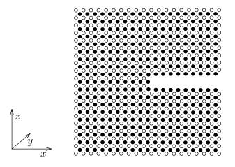
Fig. 1. Initial cavity blunting in pure bcc iron, a detail at left cavity corner
