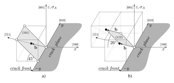
Fig. 2. Scheme of the inclined slip system  $\langle 111 \rangle \{101\}$  a) and  $\langle 111 \rangle \{112\}$  b) at the crack front
