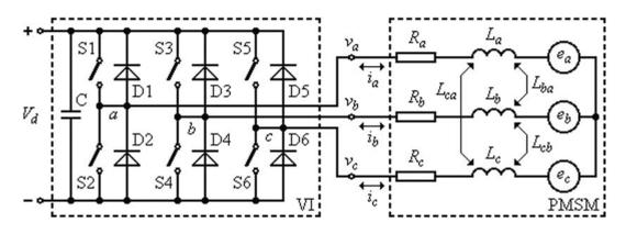
Fig. 2. Equivalent circuit diagram of PMSM and the voltage source inverter
