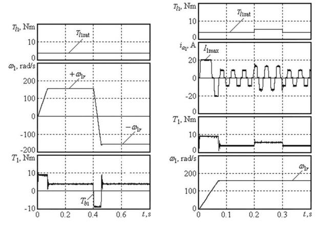
Fig. 8. Reversing with electrical breaking
