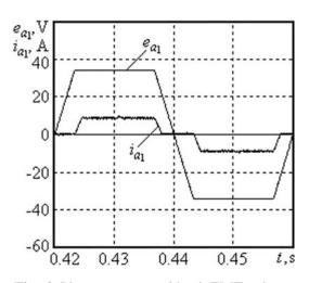
Fig. 6. Phase current and back EMF voltage
