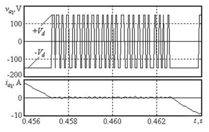
Fig. 5. Dynamic maintenance of zero phase current
