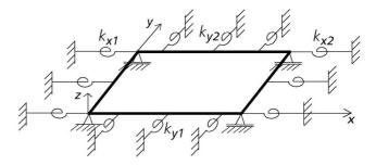
Fig. 1. Thin plate supported with torsional springs
