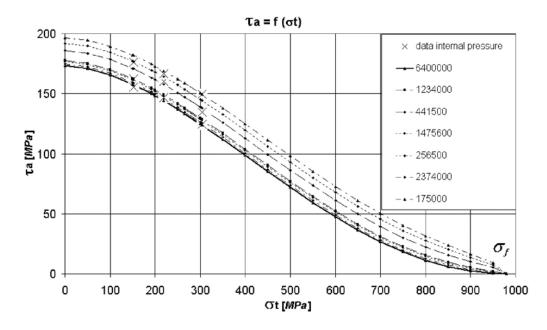
Fig. 5. Fuxa's approximation for combined torsion - inner overpressure loading
