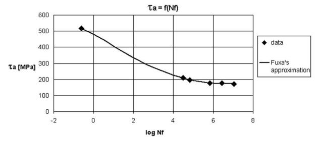
Fig. 2. S-N – curve for alternating torsion
