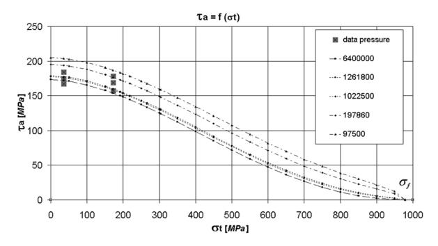
Fig. 7. The Fuxa's approximation for combined loading by torsion – inner, external overpressure and axial force
