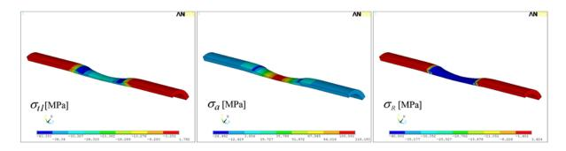
Fig. 6. Circumferential, axial and radial stresses for inner and external overpressure 40 MPa in specimen – Nr. 2. in tab. 4
