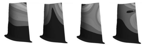
Fig. 1. First four modal shapes (displacement)
