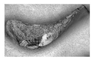
Fig. 10. Crack surface on the blade root
