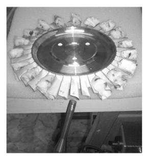
Fig. 6. Measuring system and the blisk with damped blades
