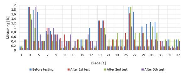
Fig. 12. Natural frequencies during testing
