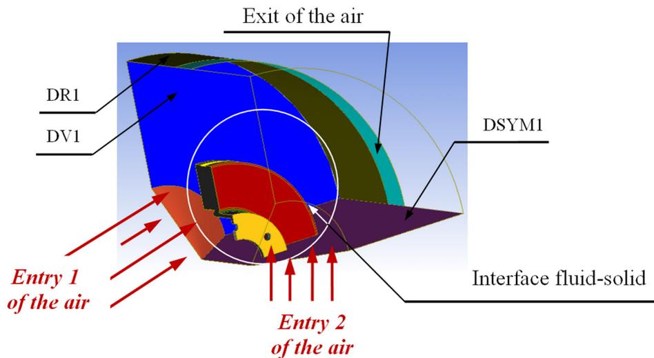
Fig. 4. Definition of surfaces of the fluid field
