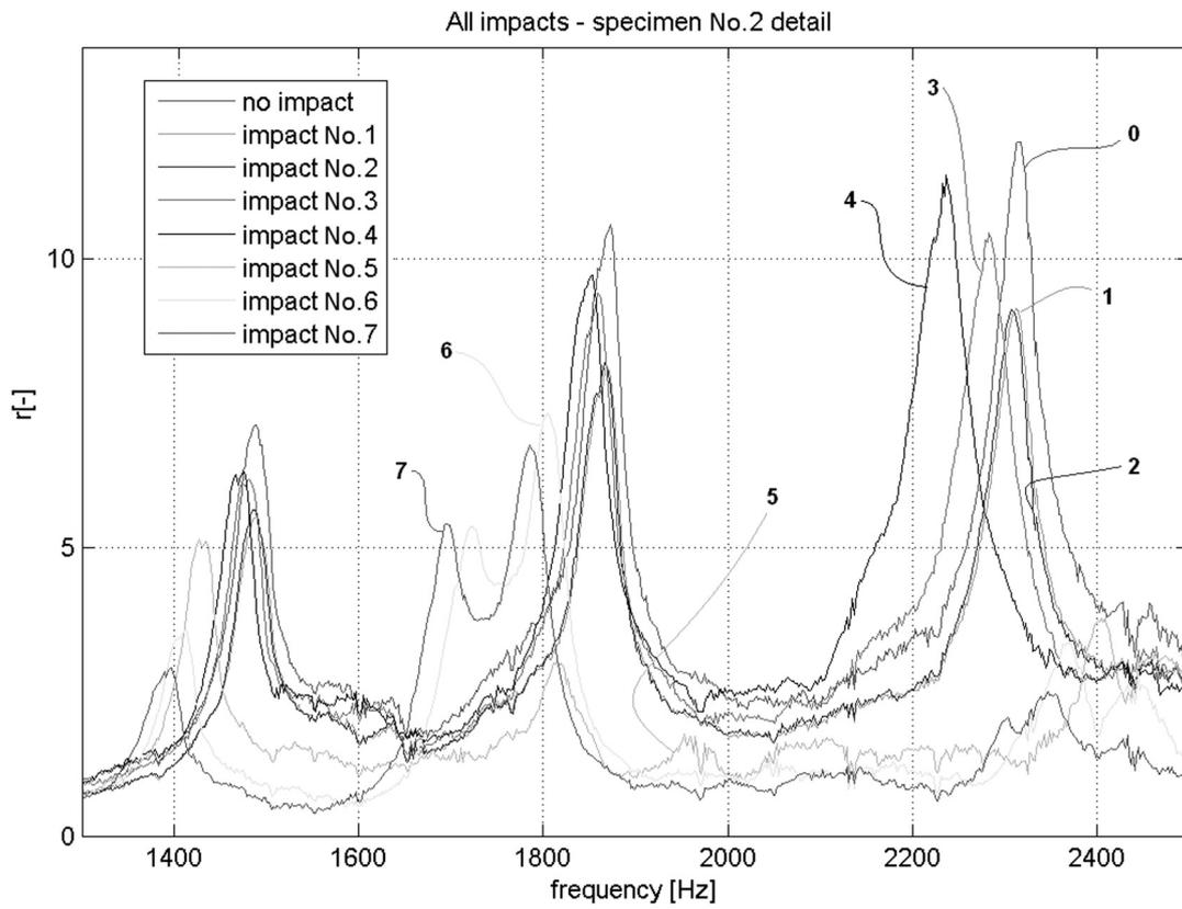
Fig. 8. Excitation after all impacts – detail – specimen No. 2
