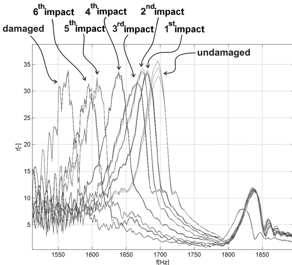
Fig. 5. Detail of shifting eigenfrequencies
