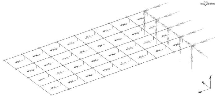
Fig. 1. Finite element model with fiber orientation in direction of arrows in elements
