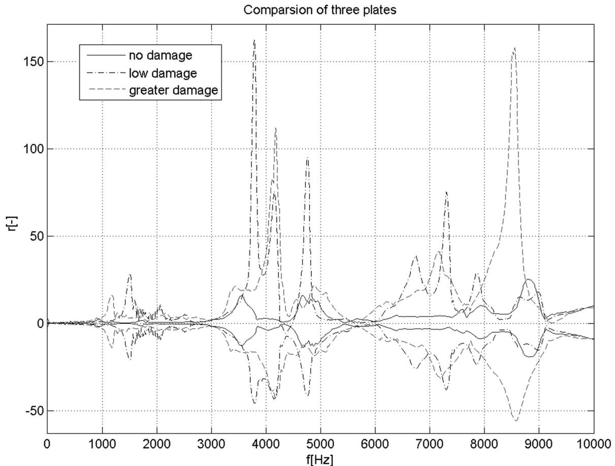
Fig. 4. Dependency of amplitude on frequency for a plate hanged on a tape
