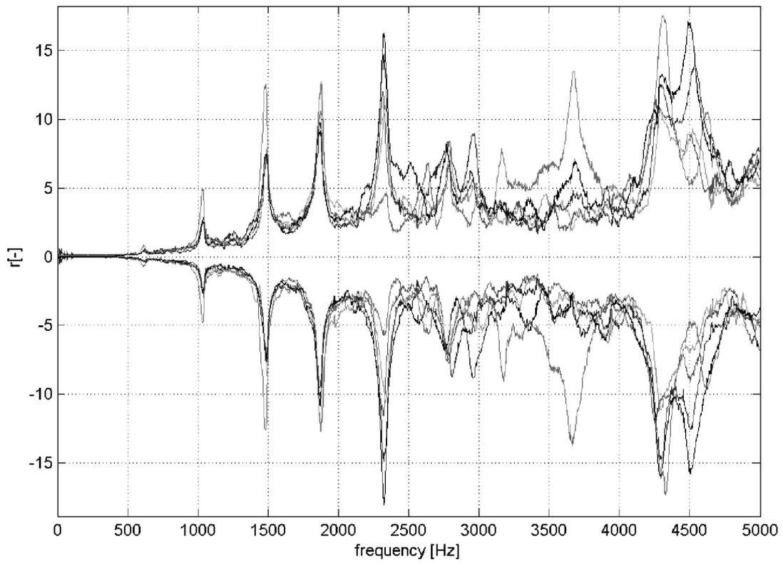
Fig. 6. Excitation with chirp before the impacts – all specimens
