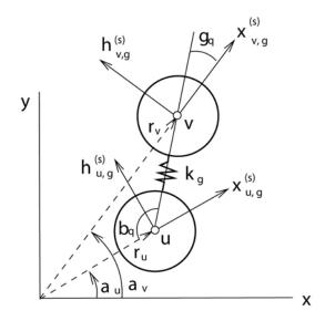
Fig. 4. The coupling between two fuel rods
