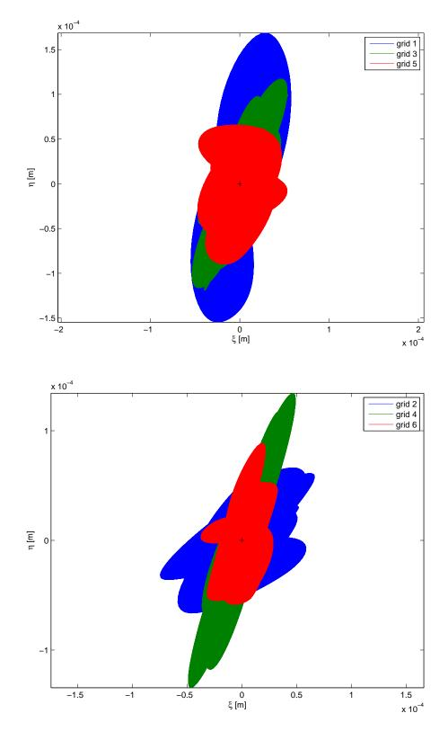
Fig. 5. Orbits of the fuel rod centre r = 10 in the first rod segment on the level spacer grids 1, 3, 5 (upper figure) and 2, 4, 6 (lower figure)
