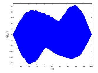
Fig. 7. Dynamic force transmitted by maximal loaded spacer grid cell (coupling 147, spacer grid 1)
