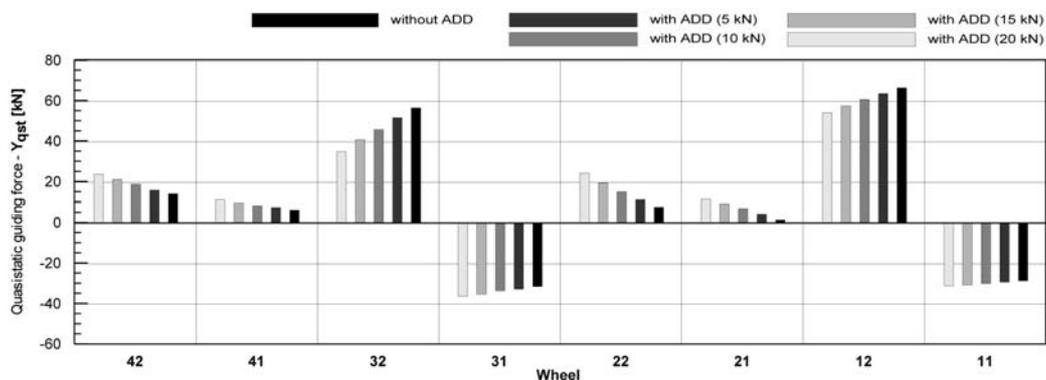
Fig. 6. Quasistatic guiding forces acting on constituent wheels in curve with radius  $R = 300$  m for value of friction coefficient in wheel/rail contact  $f = 0.40$  and for various setting-up of maximum force generated by active yaw dampers
