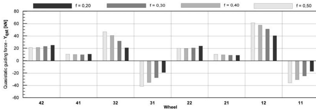
Fig. 7. Quasistatic guiding forces acting on constituent wheels in curve with radius  $R = 300$  m for value of force generated by active yaw dampers  $F_{act} = 15$  kN and for various values of friction coefficient in wheel/rail contact
