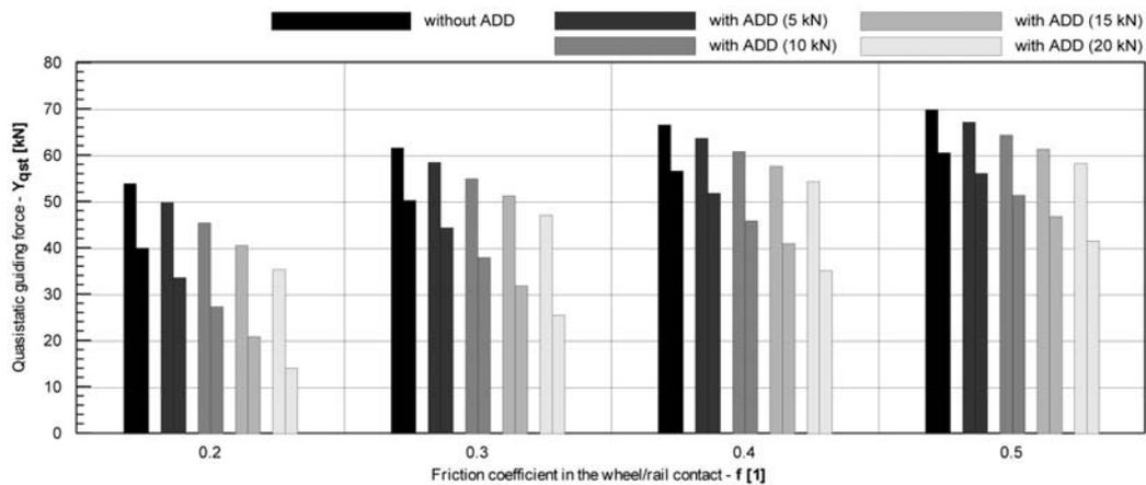
Fig. 5. Quasistatic guiding forces acting on outer wheels of the 1<sup>st</sup> and 3<sup>rd</sup> wheelset in curve with radius  $R = 300$  m for various values of friction coefficient in wheel/rail contact and for various setting-up of maximum force generated by active yaw dampers
