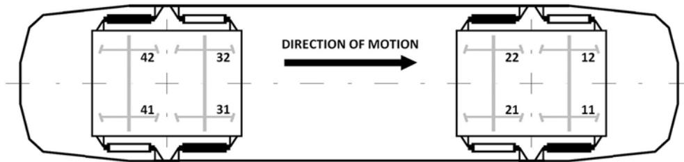
Fig. 4. Considered arrangement of classic (white) and active (black) yaw dampers on the locomotive
