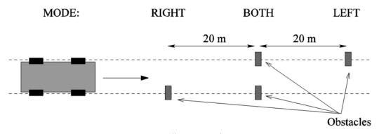
Fig. 4. Scheme of the track according to the ŠKODA VÝZKUM road vehicles testing methodology
