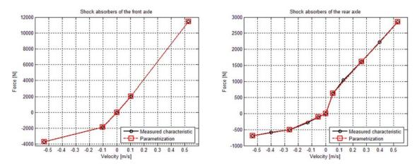
Fig. 3. The force-velocity characteristics of non-controlled shock absorbers of the front and rear axles of the SOR C 12 intercity bus and their parametrization
