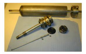
Fig. 1. The air-pressure-controlled hydraulic shock absorber and its structural members
