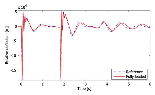
Fig. 8. Time histories of relative deflections of the right front air spring of the fully loaded bus and of the bus of the reference load (comparison of the reference case with the original force-velocity characteristics)
