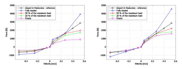
Fig. 12. The originally designed [12, 14] and the verified force-velocity characteristics of the APCSA of the rear axle of the SOR C 12 intercity bus
