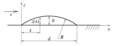
Fig. 5. The standardized artificial obstacle
