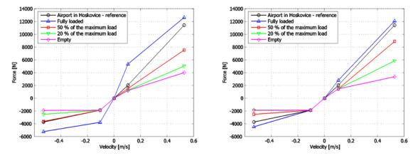
Fig. 11. The originally designed [12, 14] and the verified force-velocity characteristics of the APCSA of the front axle of the SOR C 12 intercity bus
