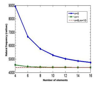
Fig. 5. The second natural frequency of rotating fixed-free tapered composite beam ( $\gamma = 10$ )
