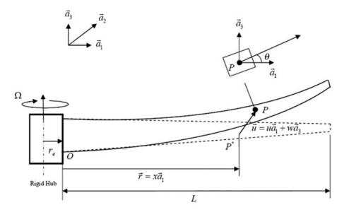
Fig. 1. Configuration of a rotating tapered cantilever beam
